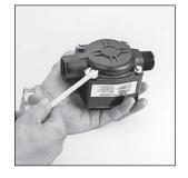
2. Tap the screws with a hammer to loosen the coverplate from the housing. (Figure 3) Remove the screws and washers.
