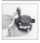
3. Gently pry the coverplate from the housing. Take care not to damage the coverplate, housing, or O-ring. (Figure 4)
