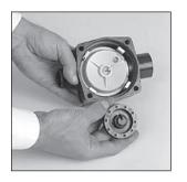
Gently remove the metal clips holding the nutator in place. (Figure 6) Take care not to damage the O-ring on the nutator inlet.
