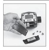
Remove the battery and, if necessary, clean corrosion from the battery terminals. (Figure 9) To prevent corrosion from condensation, coat the terminals with petroleum jelly.
