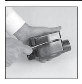
4. Remove the signal generator from the pin on the nutator disc. (Figure 5)
